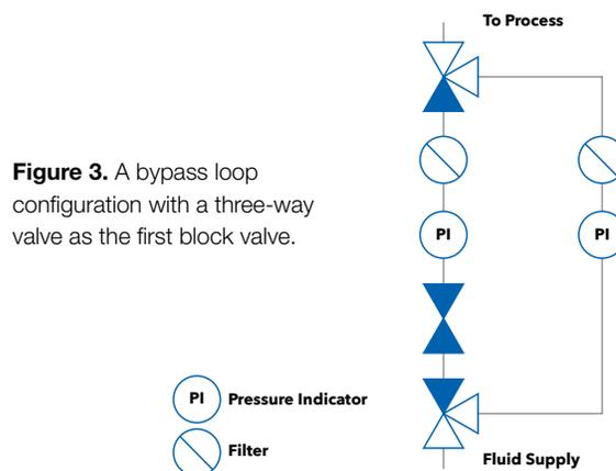
**Figure 3.** A bypass loop configuration with a three-way valve as the first block valve.
