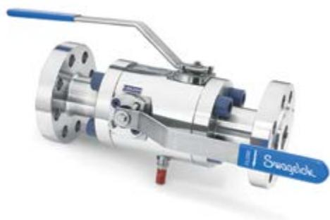
**Figure 2.** A process interface valve consolidates three valves into one valve body – two ball valves used for isolation and one needle valve for a vent.
