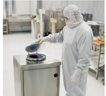
Cambridge NanoTech's atomic layer deposition (ALD) systems feature precise, controlled delivery of precursor gas to reduce gas use and thereby cost of ownership for users in the semiconductor industry and other fields.
