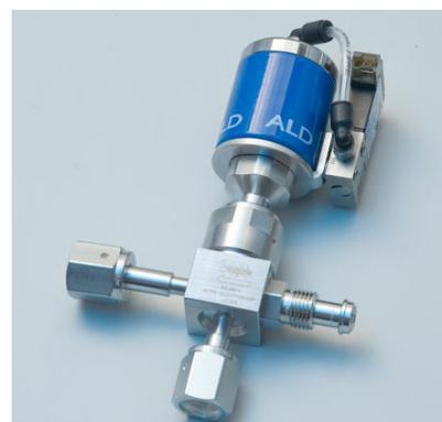
Within the ALD valve, carrier gas enters through one port and exits through another. The precursor enters through a third port, which is a small, precise orifice that delivers minimum chemical volume.
