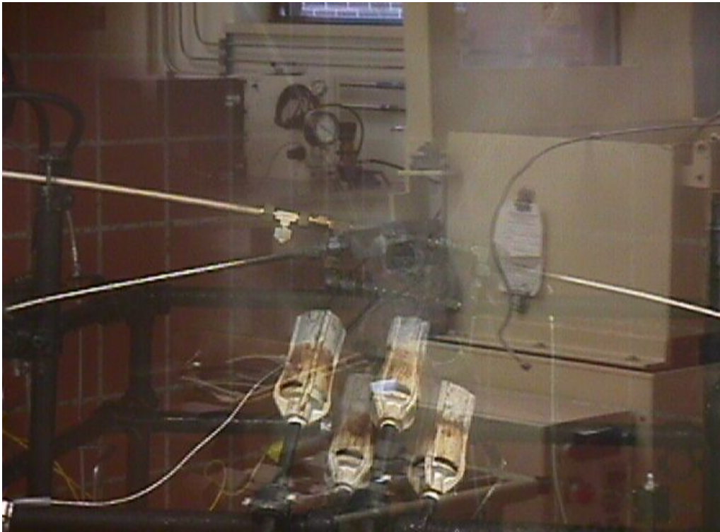
Figure 2: Samples during water quench.
