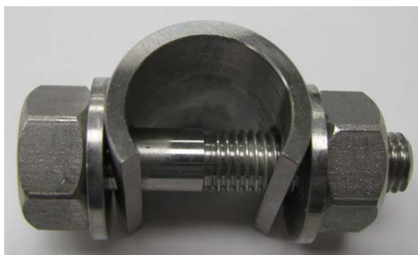
Figure 1. Test assembly consisting of C-ring, 1/4-28 bolt, nut and washers all machined from SAF 2507 super duplex stainless steel.
