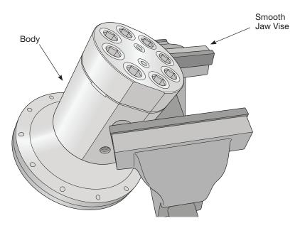
2. Loosen and remove the eight **M16 cap head bolts** by using a 14 mm hex drive.
