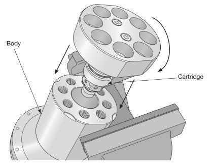
10. Insert the eight **M16 cap head bolts** by using a 14 mm hex drive torqued to 110 N·m.
