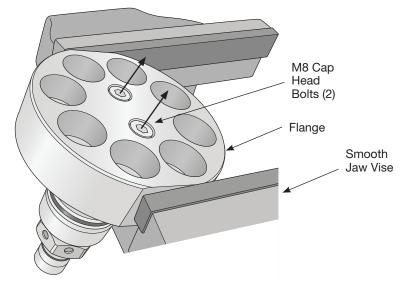
6. Remove the **cartridge** from the lower **flange**.
