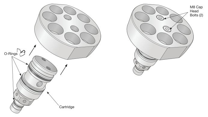
8. Hold the **body** in the **smooth jaw vise;** ensure that the internal bore is clean and free of damage. Apply lube to cartridge and body bore if required.
