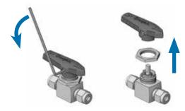
Line up the large stem flat on the valve with the large flat on the stem extension. Then slide the stem extension down onto the valve stem.
