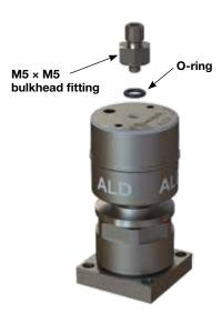
Install the O-ring into the groove of the M5 x M5 bulkhead fitting. Assemble the M5 x M5 bulkhead fitting assembly to the actuator cap and tighten between 5 to 15 in.·lb (0.5 to 1.6 N·m).
