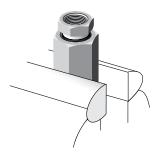
3. Remove the gland nut using an open-end wrench.
