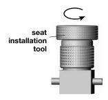
5. Remove the **seat installation tool** and **installation nut** from the body.
