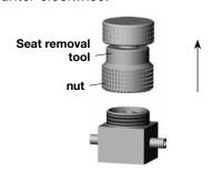
5. Turn seat removal tool to expose seat.
