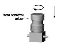
Remove seat removal tool from body by rotating nut counter-clockwise.
