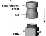
2. The **nut** should be fully tightened onto body with a **gap** showing between **nut** and **seat removal arbor.**
