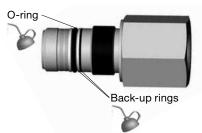
8. Lubricate the seat and end screw threads lightly with the provided MS-LT-WL7 lubricant.
