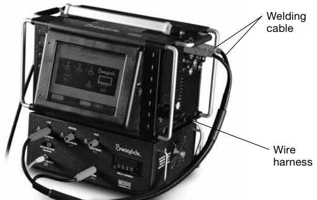
Fig. 1 – Set-up Connections
