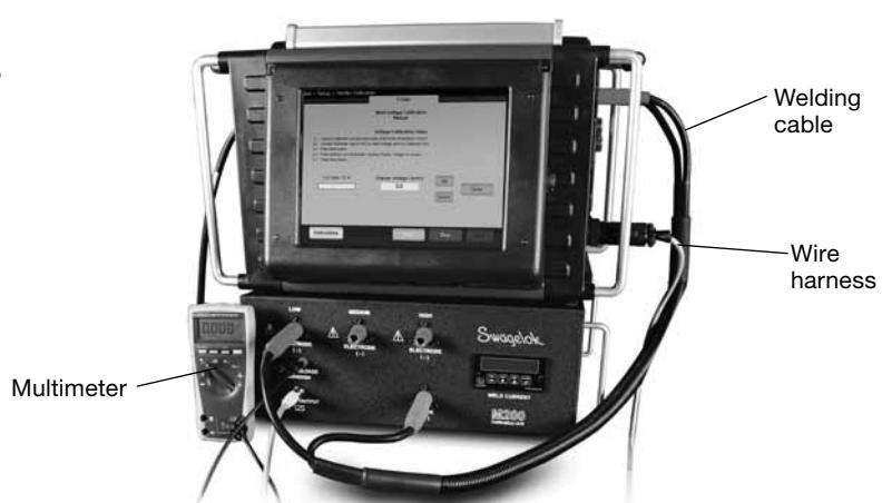
Fig. 7 — Voltage Calibration Connections
