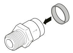
Select the trip point label that matches the replacement spring. Place the label on the identification ring.
