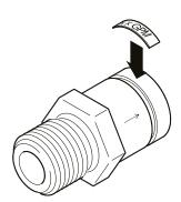
10. Thread the outlet and inlet bodies together.
