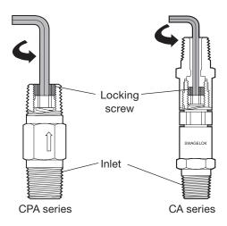
2. Slide hex wrench down into adjusting screw.
