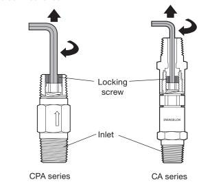
5. Verify cracking pressure.
