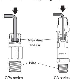
3. Turn both screws clockwise to increase cracking pressure, counter-clockwise to decrease.
