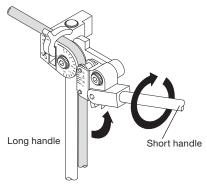
Continue the bend until the 0 on the roll support reaches the desired degree mark on the name plate.
