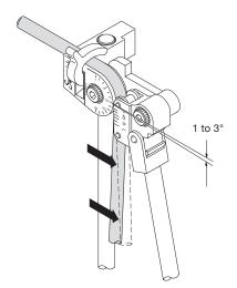
Note: Do not bend all the way to the bend mark when bending softer tubing such as copper or aluminum.
