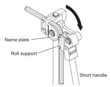
Loosen the short handle from the clevis until the short handle will swing without moving the roll support.
