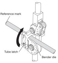
Carefully lower the short handle until the roll dies rest gently on the tube while keeping the link straight and parallel to the long handle.
