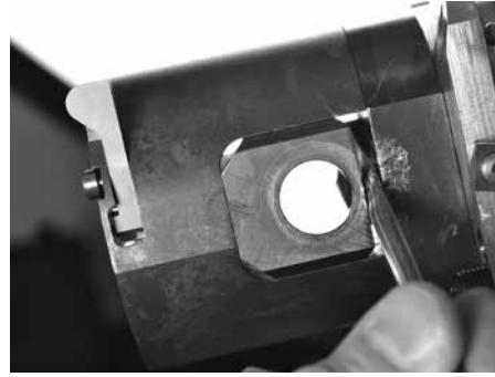
Fig. 22 Applying Lubricant to Connector Shaft
