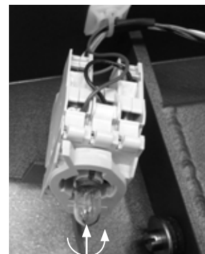
Fig. 27 Push and twist bulb CCW to remove.
