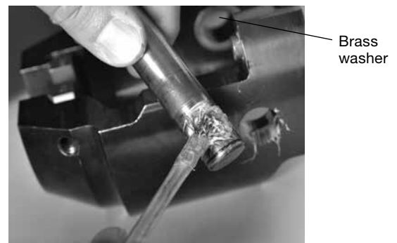
Fig. 21 Applying Lubricant to Retainer Shaft
