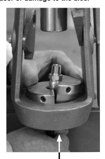
12. Remove one **die** from the **housing** while holding the **swaged assembly**. Remove the swaged assembly through the bottom of the housing.
