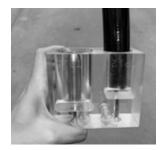
Mark the hose with a sharp grease pencil as close to the gauge as possible.
