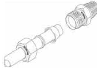
4. Insert the **tubing** into the **die head**. Make sure that the tubing rests firmly on the shoulder of the die head.
