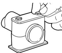
Step 5. Insert the hex-head bolts through the cover plate and body assembly. Tighten until finger-tight.
