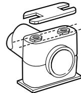
Step 3C - Align stacking bolts until hex flats can receive lock plate.
