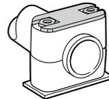
Step 3D - Place the lock plate over the body assembly and the stacking bolts.
