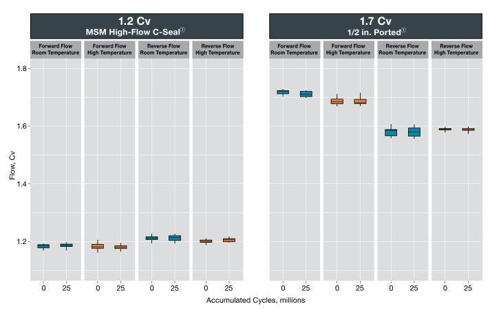
① Quantities tested: (27) MSM High-Flow C-Seal and (9) ½ in. Ported valves.
