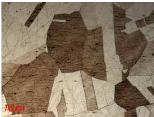
Fig. 4 Typical Microstructure of Solution-annealed Alloy 254 Forging
