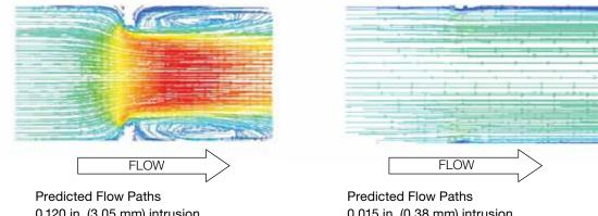
0.120 in. (3.05 mm) intrusion 5.5 inlet ft/s (1.67 m/s) velocity
