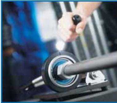
**1** Preswage the Swagelok nut and ferrules onto the tube using the multihead hydraulic swaging unit;
