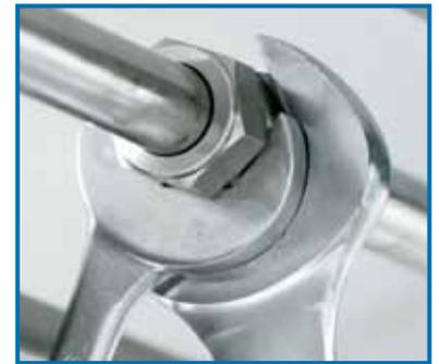
**3** turn the nut hand-tight, then tighten one half turn with a wrench.
