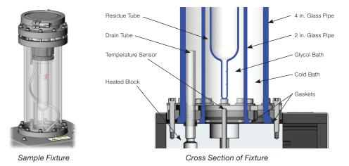
As shown, a PVC cap assembly is fitted to the residue tube to assist with the filling process. When dispensing the sample, the ammonia fills the residue tube until the level reaches the bottom of the included overflow tube. At that point, the gas trapped in the top of the residue tube prevents it from filling any further. The overflow spills into the cold bath, ensuring a consistent sample size.
