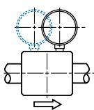
Only one gauge with a 50 mm (2 in.) or larger dial size fits directly into the body.
