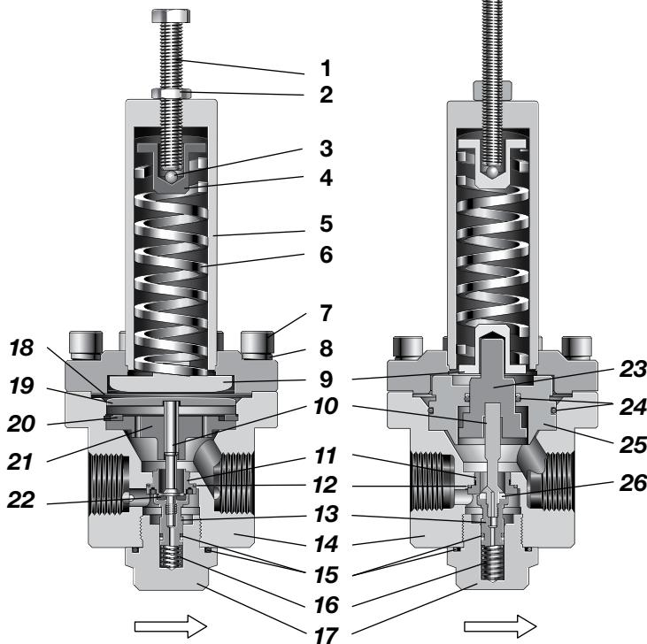
**RSH Series Regulator with Piston Sensing and Hard Seat Seal**
