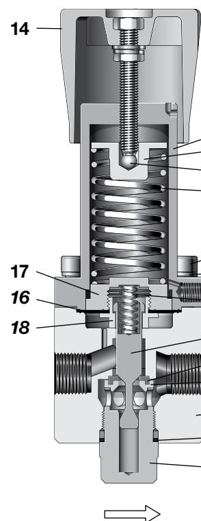
**BSH Series Regulator with Piston Sensing and Antitamper Option**
