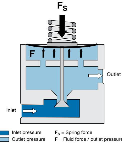
The function of a pressure-reducing regulator is to reduce a pressure and to keep this pressure as constant as possible while the inlet pressure and the flow may vary. This is accomplished by the fluid force (F) being equal to or slightly lower than load force ( $F_S$ ) causing the poppet to open.
