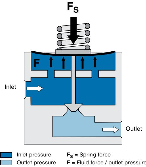
The function of a back-pressure regulator is to keep inlet pressure below a set pressure. This means the regulator can either **open** in case of excess pressure or **close** when the pressure drops below a desired pressure. This is accomplished by the fluid force (F) being equal to or slightly lower than load force ( $F_S$ ) causing the poppet to close.
