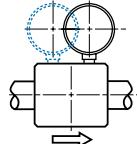
Only one gauge with a 50 mm (2 in.) or larger dial size fits directly into the body.
