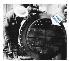
Tube plugs driven into leaking tubes into operation.
