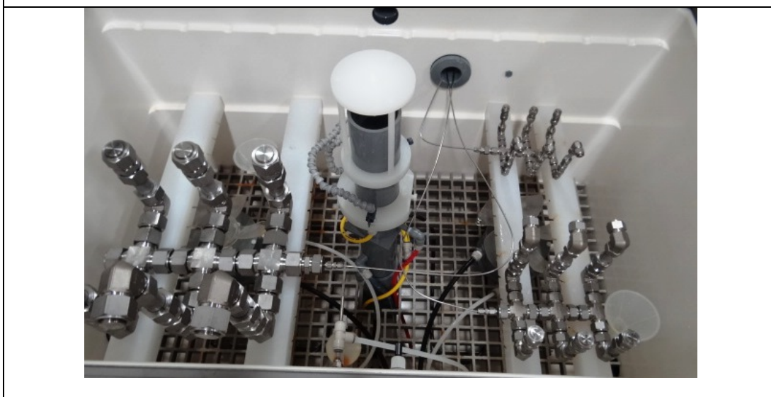
Assembled and Pressurized Tube Fittings Installed in Cyclic Salt Spray Chamber
