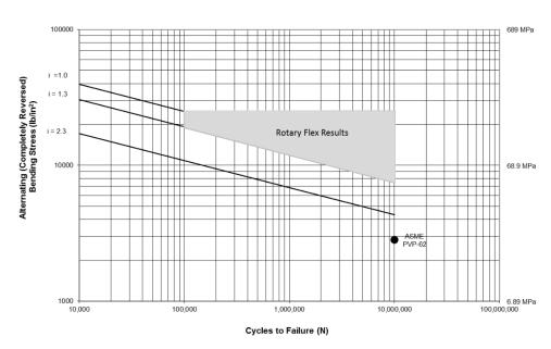
ASME B31J, Standard Test Method for Determining Stress Intensification Factors (i-Factors) for Metallic Piping Components, recommends reporting the average stress intensification, i, factor from several tests. The average stress intensification factor for the alloy 825 tubing with the stainless steel Swagelok tube fitting is i = 1.0.
