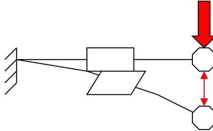
Computing an equivalent PGA seismic driver that could induce these elevated levels of shock acceleration starts with Equation 3 which relates the system resonance amplification of vibratory acceleration at an installed tube fitting as a function of driving frequency and tube system harmonic properties [ref 14].
