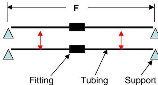
Table vibration tests were performed at room temperature under laboratory conditions at the Southwest Research Institute facilities [ref 7] in accordance with ASTM F1387 [ref 8]. The setup used in the testing is shown in Figure 1. The length “F” between tube supports (also from ASTM F1387) and the tube fitting test pressures, during and after vibration testing, for each size tube fitting were specified as shown in **Table 2**.
