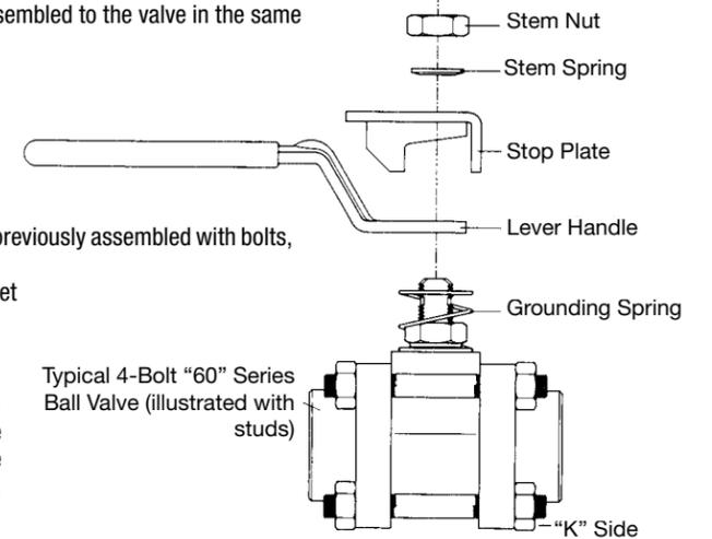
Typical 4-Bolt "60" Series Ball Valve (illustrated with studs)
