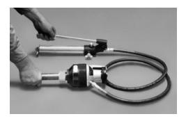
Swagelok hydraulic swaging units preswage 1/2 to 2 in. and 12 to 38 mm Swagelok ferrules onto carbon steel and stainless steel tubing prior to assembly into a Swagelok tube fitting.
