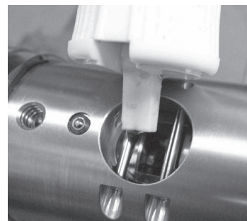
Fig. 35 Applying cutting fluid to coning blade, manual adapter and end of tube
