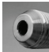
Acceptable ID of the nipple properly deburred.
