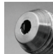
Non-conforming burrs present in ID of the nipple. Note: Image shows a cone ID that has not been deburred and tearing is shown on the cone.
