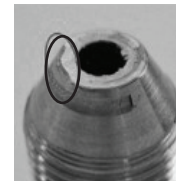
Non-conforming damaged cone face diameter dropped.
