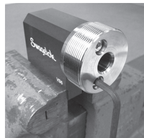
Fig. 2 Removing/Attaching the manual adapter
