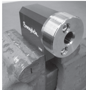
Fig. 17 Placing the tube vise in a bench vise
