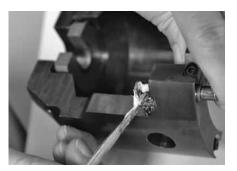
Fig. 23 Applying Lubricant to Latch Pins
