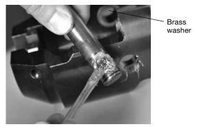
Fig. 21 Applying Lubricant to Retainer Shaft
