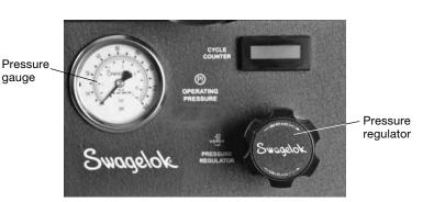
Fig. 12 Front Panel of HVSU
