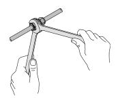
Fig. 16 Tighten Nut with Wrench
