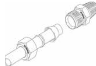
Nut and ferrule in the correct order on the tubing
