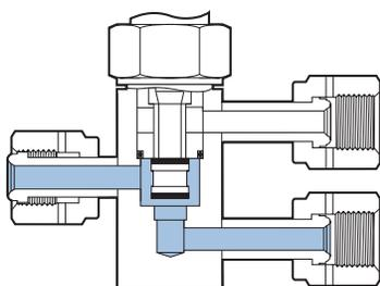
When there is no pressure to the actuator, the stem tip seals the lower port, allowing flow through the upper port.
