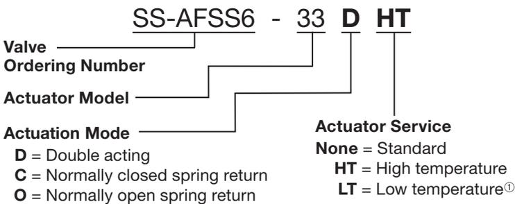
For dual-mounted assemblies (two valves mounted to one actuator), add **DM** to the ordering number. Example: SS-AFSS6-33DHTDM
