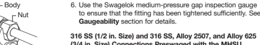
4. Place a mark on the fitting **body** in line with one of the hex points of the **nut**.
