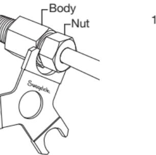
Swagelok medium-pressure gap inspection gauge
