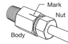
5. Hold the fitting body steady and tighten the nut one-third turn. This is equivalent to advancing the nut two hex points from the scribed mark.
