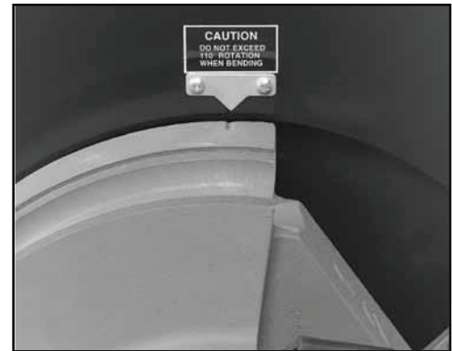
Figure 6 1 and 1 1/2 in. (25 and 38 mm) Reference Notch
