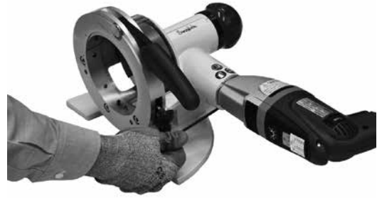
Fig 16 Loosening the Set Screw
