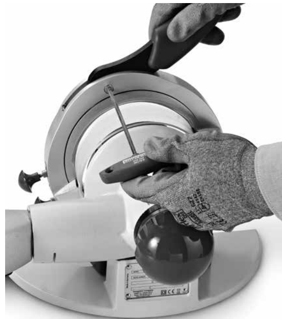
Fig 13 Loosening the Socket Screw
