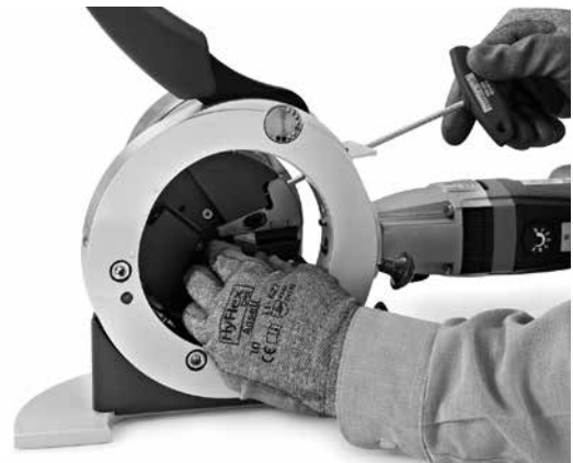
Fig 7 Installing the Tool Holder
