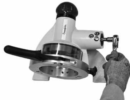
Fig 18 Removing the Breakaway Nut
