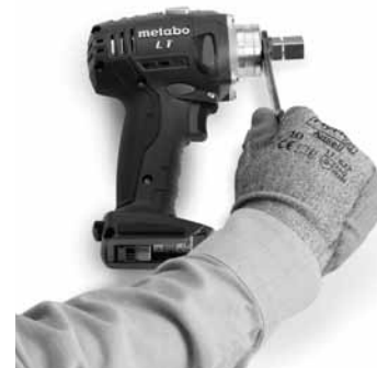
Fig 34 Removing the Breakaway Nut
