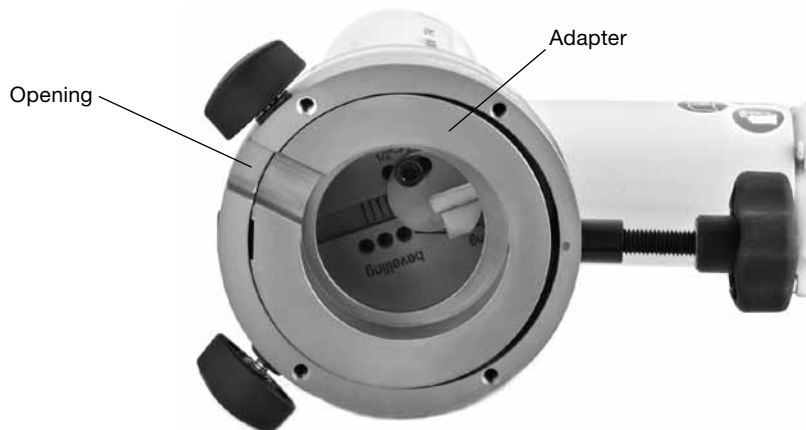
Fig 23 Inserting the Collet Set Adapter
