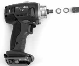
Fig 35 Breakaway Nut Removed from Tool
