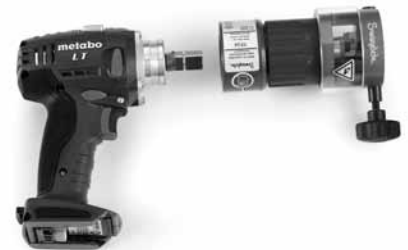
Fig 33 Removing the Collet Housing Half of Tool
