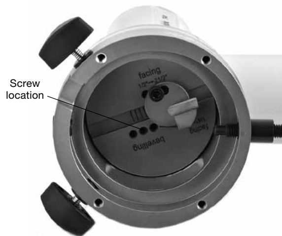
Fig 14 Installing the Tool Holder, TF40 series
