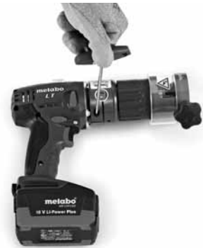
Fig 32 Loosening the Set Screw
