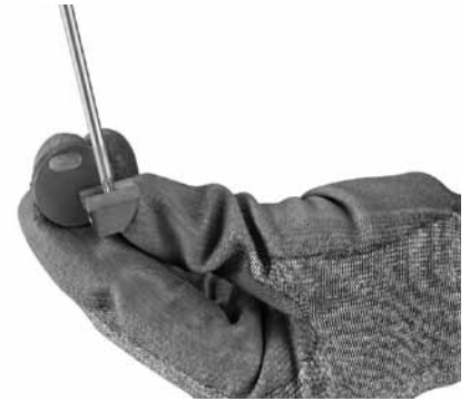
Fig 12 Installing the Cutting Insert
