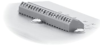
Terminal Strip Proximity Sensor Interface (shown enlarged, without sealed enclosure)
