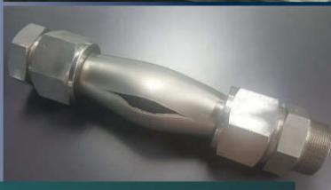
Swagelok fittings are subjected to extreme burn, rotary flex, impulse, corrosion, and shock impact testing; some tests take as many as 10 million cycles to complete
