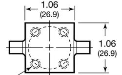
Four mounting holes, M5 × 0.8-6H thread, 0.25 (6.4) deep, located 45° from center line, on a 1.00 (25.4) bolt circle. M5 × 0.8-6H holes are compatible with 10-32 mounting screws.
