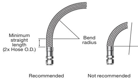
Hose rupture or leakage may result from bending too close to the hose/fitting connection.
