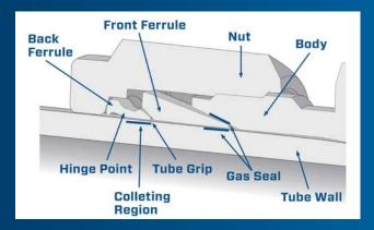
SAT12 is Swagelok's unique low-temperature carburization process. It achieves a phenomenal tool steel-like hardness and strength in the ferrule without sacrificing corrosion resistance or material ductility (is non-brittle). In use for nearly two decades, it enriches the surface of stainless and other metal alloys by diffusing carbon atoms between metal atoms without forming carbides.
