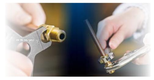
Practical: Calculate, cut, measure, bend tubing for test loop assembly Correctly install tube fittings onto test loop Visual inspection with gap inspection gauge tool Correctly re-assembled connections
