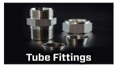
Swagelok Tube Fittings, consisting of a body, nut, and front and back ferrules, incorporates a grip-type mechanism that creates a unique hinging-and-colleting action that yields superior isolation of stress risers at the tube grip to effectively resist bending, deflection, and vibration.
