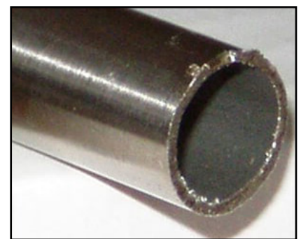
Tubing not properly deburred.
