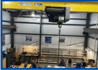
5-ton Overhead Crane, with 18-foot clearance
