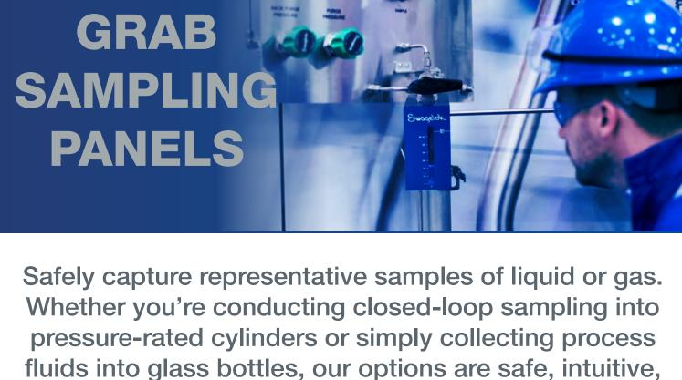
Offered in 8 standard Grab Swagelok Sample Module (GSM) Panel configurations that employ pressure-containing metal cylinders to provide a sample held under the same process conditions as when extracted.
