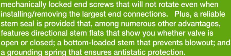
The new Swagelok® GB Series General-Purpose, Bi-Directional, Full-Flow Ball Valve will slash your installation, maintenance, and
